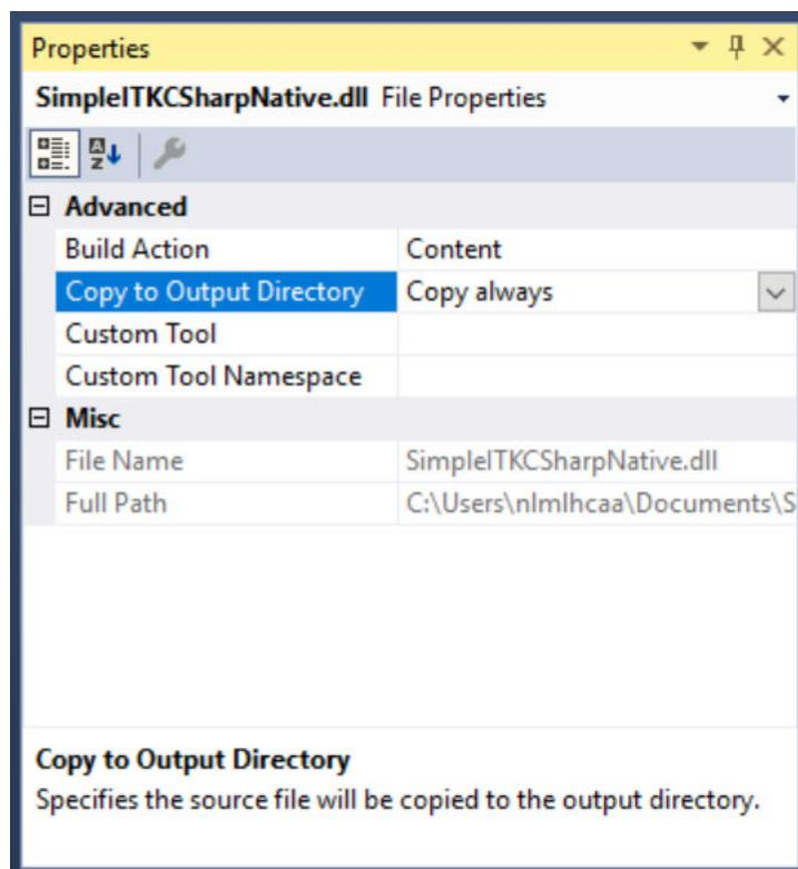
Then click *Build -> Build Solution*. Assuming you have followed all of the steps thus far, you should have an executable you can run from the command line or from Visual Studio by adding command line arguments in *Project -> ConsoleApp1 Properties... -> Debug*.
